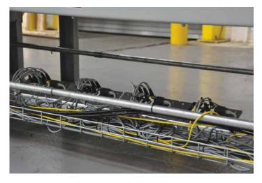
Machine wiring with SmartWire-DT
