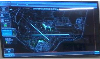
The storm warning system central control & monitoring unit not only controls the remote siren and strobes, but also monitors the operating and condition status of these — allowing for appropriate proactive preventative maintenance and for alarm warning of failures, to maximise reliability of system.
